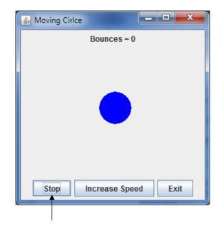
When clicked, circle moves, and text of the button changes to "Stop". Circle moves horizontally at 1 pixel per 10 milliseconds.
